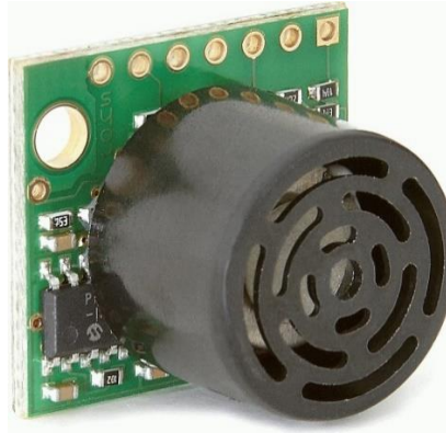
Figure 13: LV-MaxSonar-EZ0 Reprinted with permission of MaxBotix
